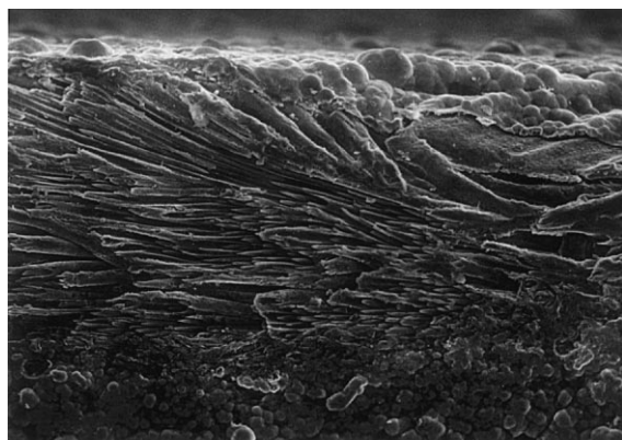
Fig. 4. Surface of N11 specimen after 10 plasma exposures; surface was oriented perpendicular to the magnetic field of TEXTOR.
